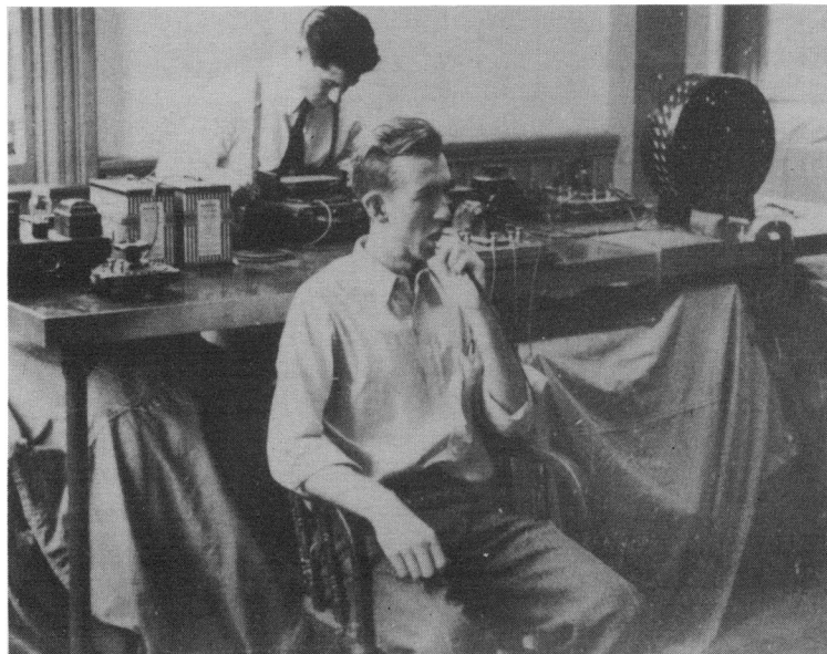
Fig. 1 - Determination of perception current on the tongue.
